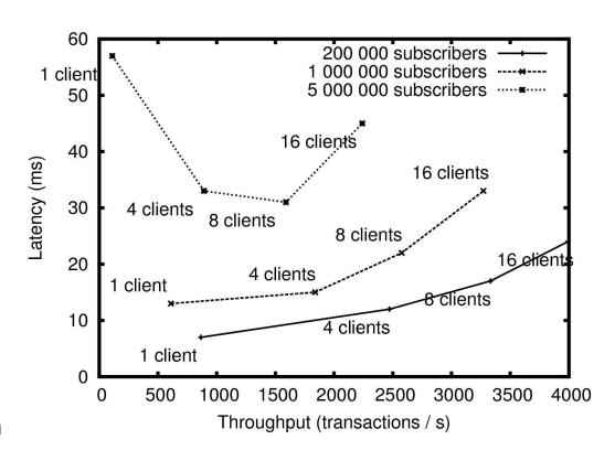
Source: R. Paivarinta and Y. Raivio: Performance Evaluation of NoSQL databases in Mobile Networks, Closer2011
